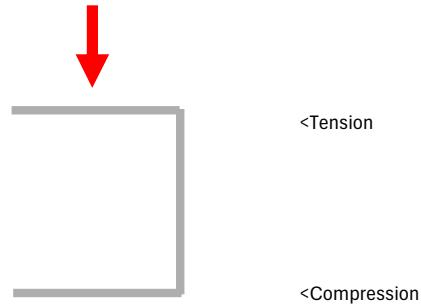
Compressive axial load at base of walls
