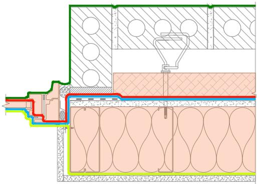
Water-Shedding Surface and Control Layers of Detail 6-10
